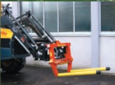
Front loader with hay bale fork With fast-changeable-mechanism for different front attachments.
